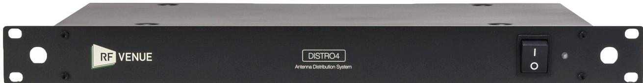
DISTRO4 is a broadband UHF antenna distribution amplifier that routes antenna signals from a pair of diversity antennas to several receivers in a multi-channel system. DISTRO4 compensates for signal strength lost in the splitting process with high quality amplifiers. Two or more units may be cascaded together to accommodate more than four receivers with the included cascade port.
